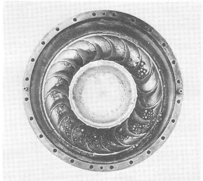
Fig. 9 Failed hydrokinetic brake toroid after blade disintegration
